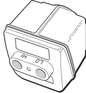
HM2-2 are high pressure measurement devices. They are single-port modules based on sensors capable of measuring gauge, absolute, compound or vacuum with ranges spanning from vacuum to 5 psi to 10,000 psi. All wetted parts are 316 stainless steel (except for 10k psi module which has 17-4ph stainless steel) and are intended for use with any pressure medium compatible with stainless steel.
