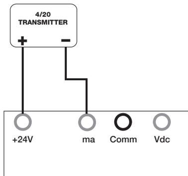
V OUT TRANSDUCER HOOK UP USING, INTERNAL SUPPLY
