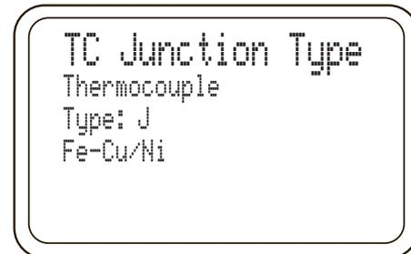
Note; By selecting the thermocouple type the PTE-2 will access the factory programmed coefficients in the module which will allow the PTE-2 to display in a unit of temperature
