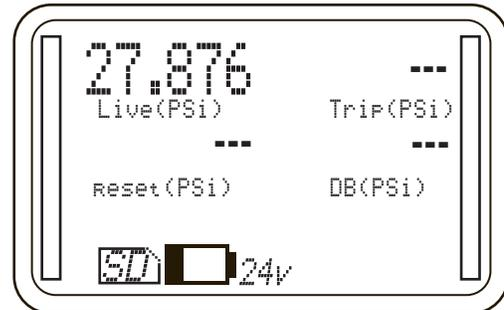
In Switch Test Mode the display will initially show the Live pressure (pressure being applied at that time), and units of measure. The switch trip point, reset point and dead band (DB) will be blank indicated by "---"
