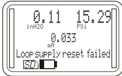
Note: A direct short between 24Vdc out and COM terminals will cause complete shut down of the base unit. Remove shorted leads and power the HHC on with the power key. Base unit will not be damaged, however warning messages will not be displayed.
